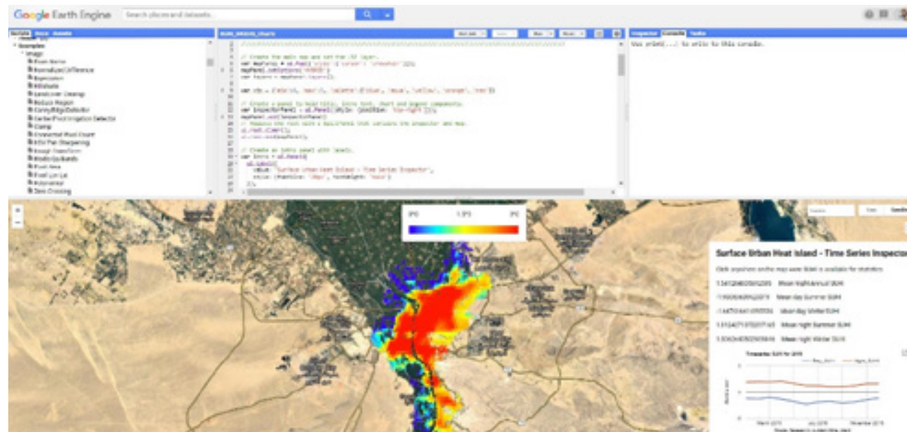
Figure 5.22. Google Earth Engine (GEE) can be used to process massive amount of EO data. The illustration shows a GEE app developed by www.rslab.gr to monitor Urban Heat Island across the whole globe using the complete archive of NASA MODIS observations, (©RSlab).
