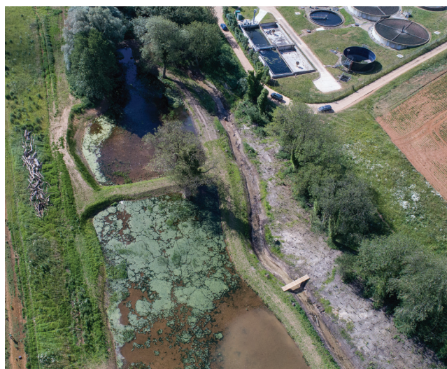
Aerial view of Ingodisthorpe recycling center with ponds forming the new treatment wetland © ANGLIAN WATER
