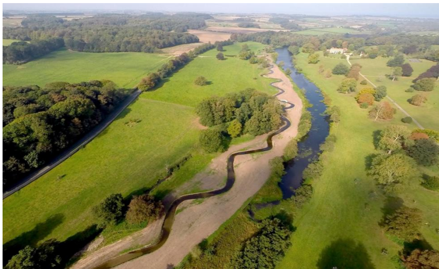
Channel re-meandering | River Glaven, Norfolk. ©Norfolk Rivers Trust
