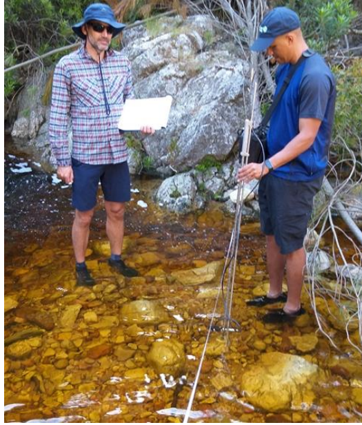
Figure 12. Streamflow discharge measurements are routinely collected at each experimental catchment during field visits.
