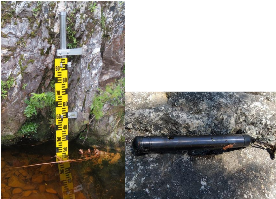
Figure 11. The stilling well and gauge plate set-up (left) used at each experimental catchment. The Solinst LTC loggers (right) are installed within the stilling well.
